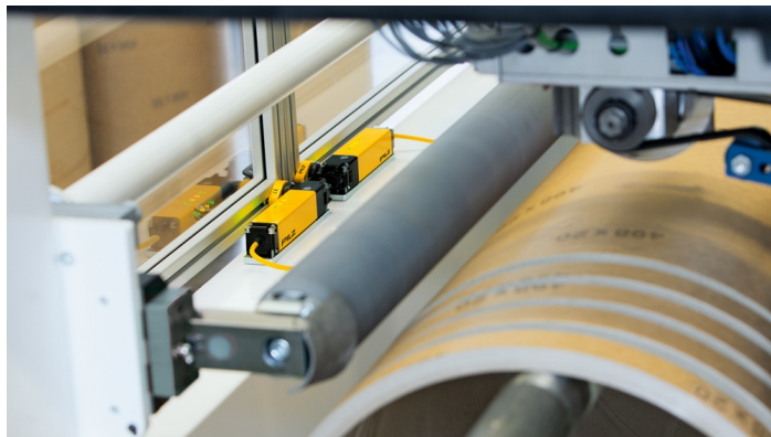
Caption: ISO 14119 specifies the design principles for the safeguarding of safety gates with interlocking switches. Now there is a new version of the standard. (Photo: © Pilz GmbH & Co. KG)
