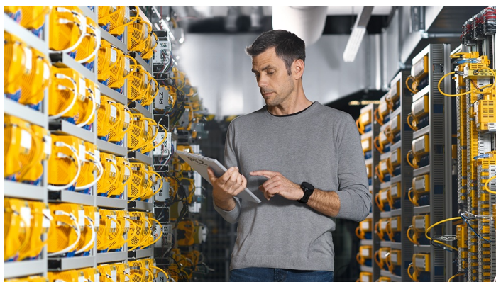
Caption: Pilz develops controllers for the safe automation of plant and machinery. In the test laboratory in Ostfildern, Pilz engineers subject PLC controllers to an endurance test. (Photo: © Pilz GmbH & Co. KG)
